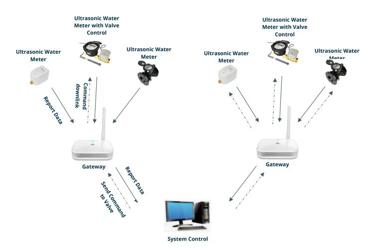
Our smart gateway receives near real-time data from all the valves within range, converts the raw data into an easy-to-use JSON format, and then publishes it using MQTT protocol. Data can be sent to any local or cloud MQTT broker via Ethernet, LTE (4G), or WIFI.
