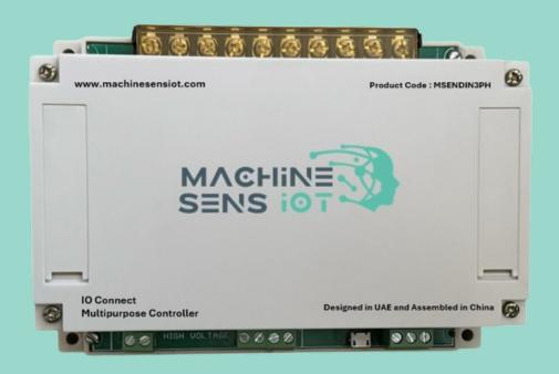
Advanced I/O & Relay controller for a wide range of automation and wireless IoT applications
